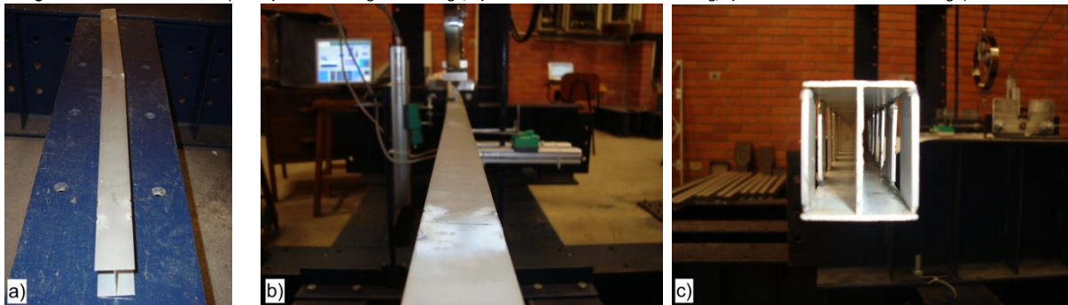
Figure 11. Modes failure examples. a) Local buckling of the flange; b) Inelastic lateral-torsional buckling; c) Elastic lateral-torsional buckling. (Self-Elaboration).
