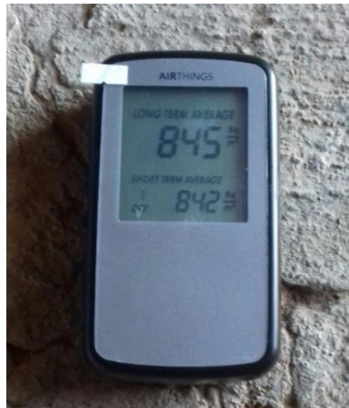
Figure 6. Measurement (Bq/m 3 ) of gas radon inside a house. Source: by the author.
