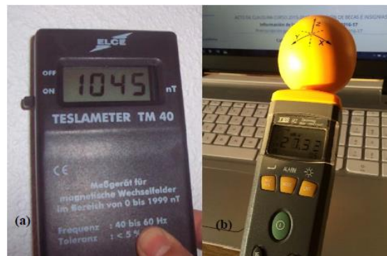
Figure 7. Measurements (nT and nW/cm 2 ) of the electromagnetic field: low frequency (a), high frequency (b). Source: by the author.
