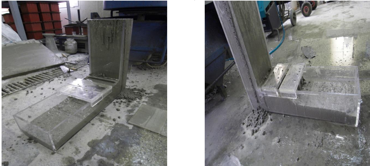
Figure 12. (a-b) L Box used in the experiments. (Self-Elaboration).
