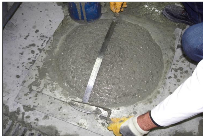
Figure 15. Spread measurement of SCCs (Gökçe, M., 2013).
