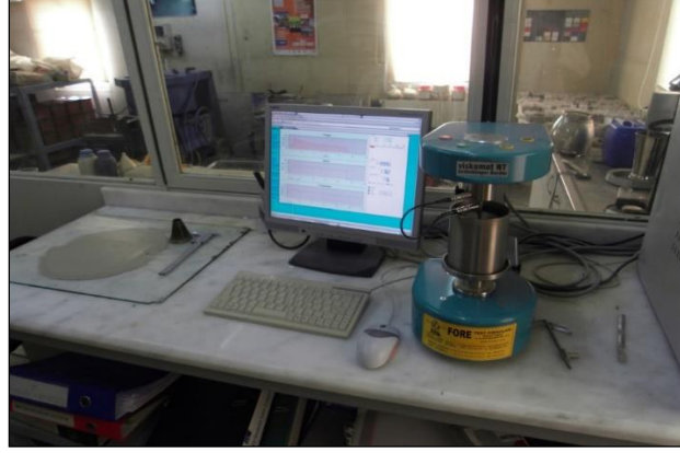
Figure 4. The testing device used to perform rheological measurements. (Self-Elaboration).
