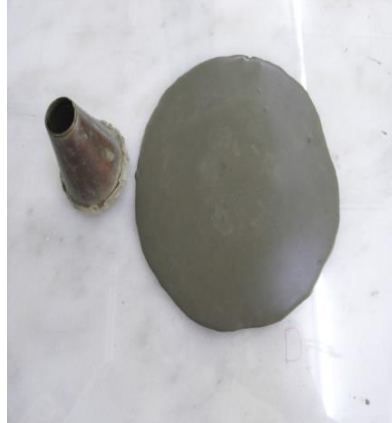
Figure 5. Mini-slump flow test (Gökçe, M., 2020).
