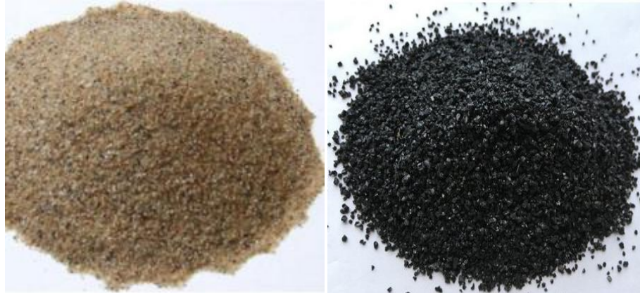
Figure 2. Visual observation (a) river sand (b) copper slag. (Self-Elaboration).
