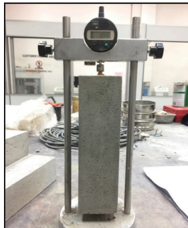
Figure 4. Instrument for drying shrinkage test
